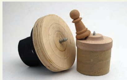
Smaller-size shopmade screw chucks provide fast and easy mounting of small projects such as chessmen (right). Use a lag bolt if more support is needed, as shown in the example on the left that uses a faceplate and a scrap of plywood.
