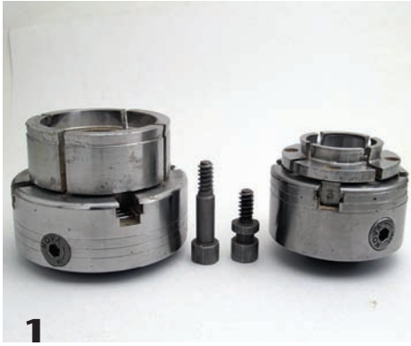
1 The screw on the left projects \frac{3}{4} " (20mm) beyond the jaws. The one on the right projects \frac{5}{8} " (16mm).
