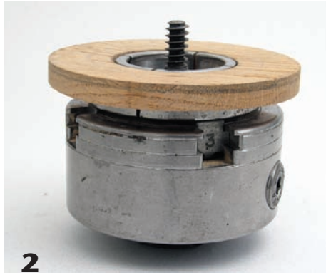
2 A large hardwood washer greatly strengthens the hold.
