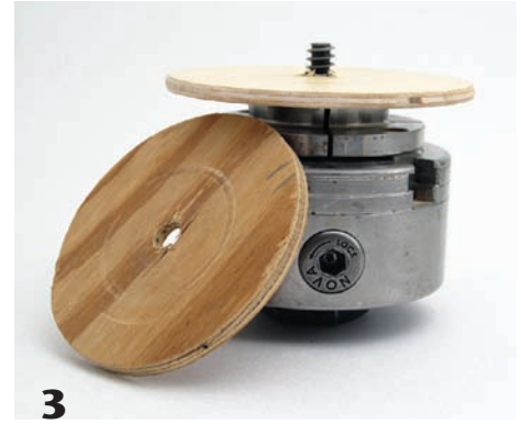
3 Use a plywood spacer when a smaller-depth hole is required.
